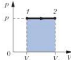
$$A = p \cdot \Delta V = p \cdot (V_2 - V_1)$$
